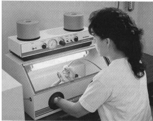
Figure 5. Microabrasive blasting workstation with partial views of dust collector (left) and air-dryer (upper right).
