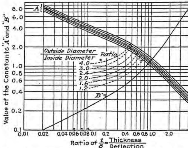
FIG. 19 CONSTANTS FOR CALCULATING INITIALLY FLAT DISK SPRINGS
