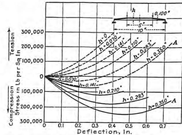
FIG. 13 COMPUTED MAXIMUM STRESSES FOR SIX DISK SPRINGS IDENTICAL EXCEPT FOR FREE HEIGHT (Solid lines show stress at upper edge of inner diameter. Dashed lines show stress at lower edge of inner diameter.)
