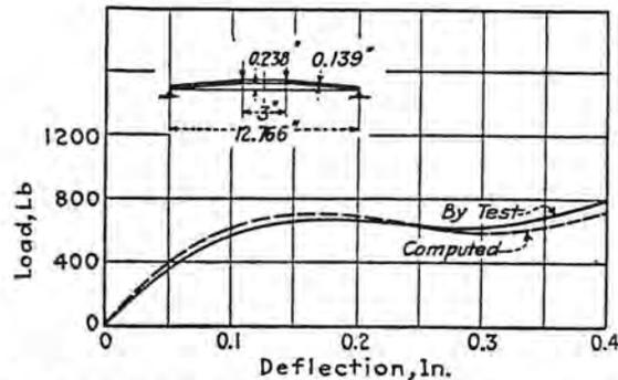
FIG. 7 LOAD-DEFLECTION CURVES OF A DISK SPRING HAVING A LARGE OUTSIDE-DIAMETER-INSIDE-DIAMETER RATIO
