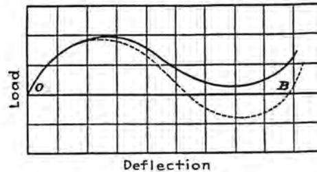
FIG. 1 GENERAL SHAPE OF A DISK-SPRING LOAD-DEFLECTION CURVE HAVING A VARIABLE SPRING RATE
