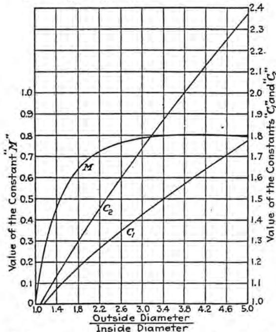
FIG. 18 LOAD AND STRESS CONSTANTS FOR CALCULATING DISK SPRINGS
