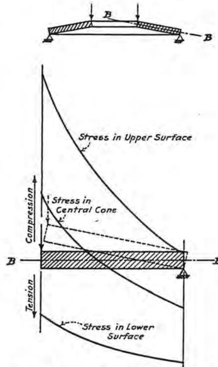
FIG. 15 COMPUTED STRESS DISTRIBUTION OVER THE WIDTH OF A DISK SPRING. SPRING OF FIG. 14 DEFLECTED TO FLAT POSITION
