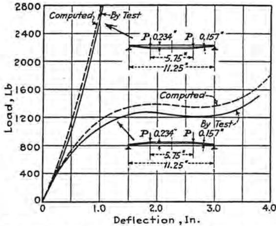
FIG. 8 LOAD-DEFLECTION CURVES OF A DISK SPRING LOADED IN TWO DIRECTIONS
