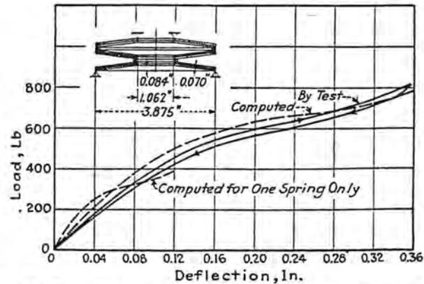
FIG. 11 LOAD-DEFLECTION CURVES AND HYSTERESIS OF SIX SPRINGS, THREE GROUPS OF TWO PARALLEL SPRINGS LOADED IN SERIES
