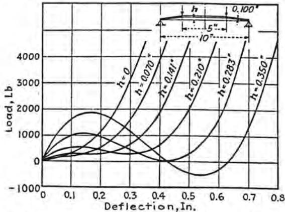
FIG. 3 COMPUTED CHARACTERISTIC LOAD-DEFLECTION CURVES OF SIX DISK SPRINGS IDENTICAL EXCEPT FOR FREE HEIGHT  $h$
