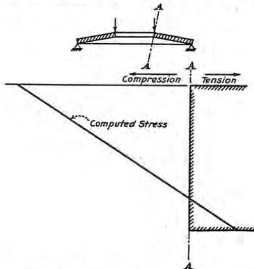
FIG. 16 COMPUTED STRESS OVER THE THICKNESS AT THE INNER CIRCUMFERENCE OF A DISK SPRING. SPRING OF FIG. 14 DEFLECTED TO FLAT POSITION
