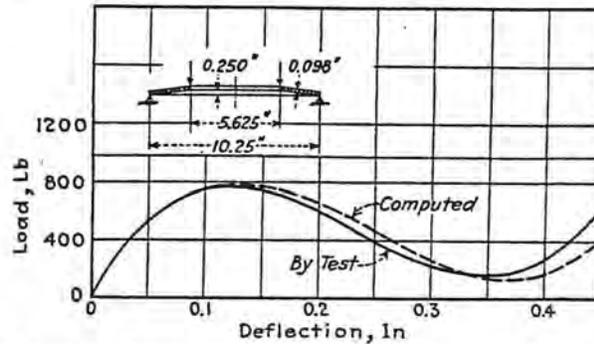
FIG. 6 LOAD-DEFLECTION CURVE OF A DISK SPRING HAVING A NEGATIVE RATE
