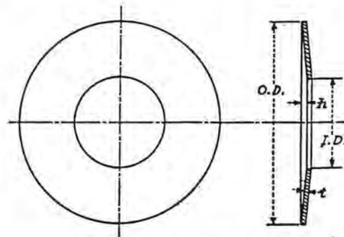
FIG. 2 ANNULAR-DISK SPRING
