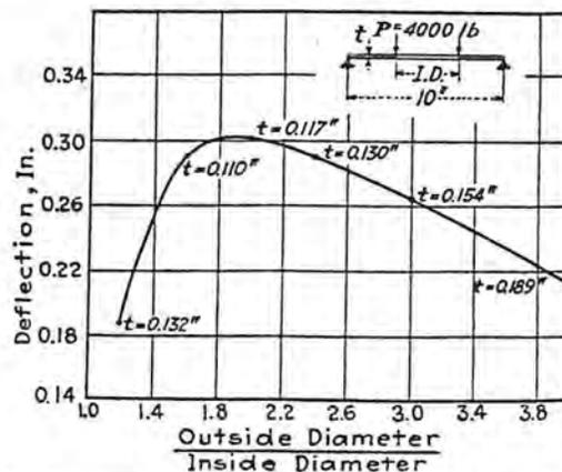
FIG. 12 INFLUENCE OF OUTSIDE-DIAMETER-INSIDE-DIAMETER RATIO ON THE FLEXIBILITY (DEFLECTION-LOAD) OF AN INITIALLY FLAT DISK SPRING UNDER 4000-LB LOAD
