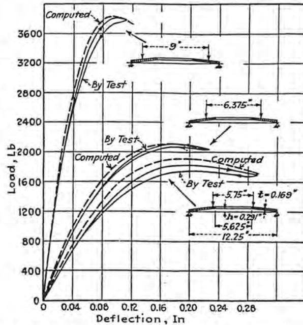
FIG. 10 LOAD-DEFLECTION CURVES OF A DISK SPRING LOADED AT VARIOUS DIAMETERS
