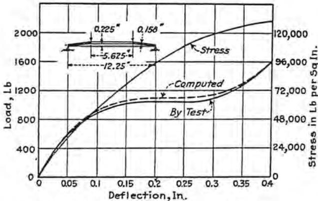
FIG. 14 LOAD-DEFLECTION CURVE OF A DISK SPRING HAVING A WIDE ZERO-RATE RANGE
