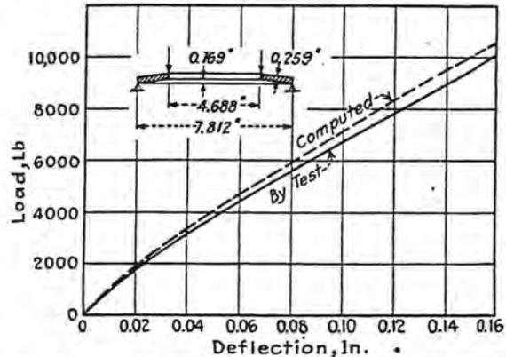
FIG. 5 LOAD-DEFLECTION CURVE OF A THICK DISK SPRING
