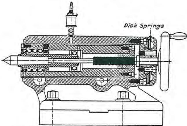
FIG. 9 TAILSTOCK CENTER WITH DISK SPRINGS
