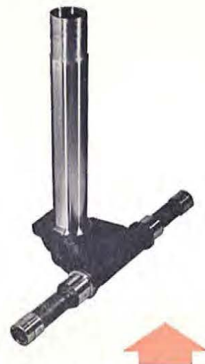
Fig. 6—Aircraft landing-gear part of ultrahigh-strength steel is shot peened to overcome effects of decarburization
