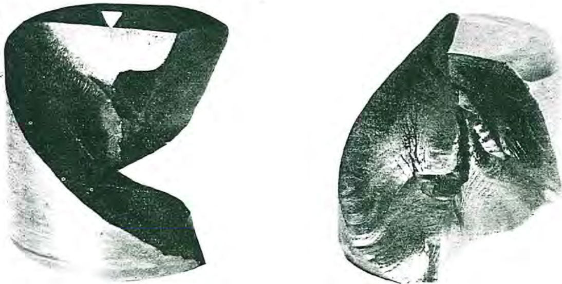
Fig. 22. "Explosive" fracture of bearing roller caused by unfavorable residual stresses
