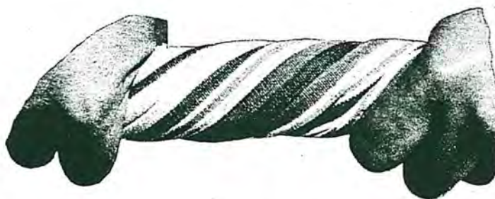
Fig. 1—Pattern of compressive and tensile stresses from torsional loading is illustrated by this analogy. Water is pressed from cloth by compressive forces acting perpendicular to the stripes. Cloth is torn by tensile forces acting in the direction of the stripes.
