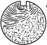
POINT OF ORIGIN AT KEYWAY GLAM SHELL FRACTURE GHARACTERISTIC OF
