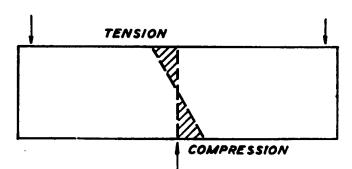
The same part, when shot peened overall in the unloaded condition, has its surface in compression due to the cold working and plastic upsetting of the surface metal by the hail of shot. Since the surface is in compression, the core is in tension to balance out the forces as shown in following diagram:
