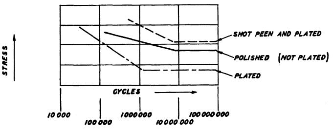
peening; however, shot peening will not improve a decarburized part to the point where it is as good as a properly heat treated part.
