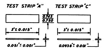
These strips of SAE1070 cold rolled spring steel are heat treated to 44-50  $R_c$ . and must have a flatness of .0015 arc height as measured on the Almen Gage. It should be noted that practically all test strips purchasable today are about 46-48  $R_c$ , and within 0.0005 arc height.
