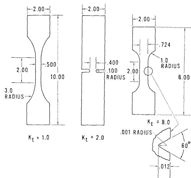
Fig. 1—Configuration of sheet specimens
