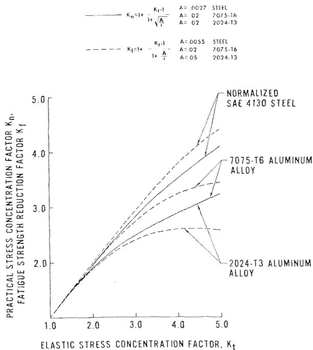
Fig. 5—Stress-concentration factors for edge notches
