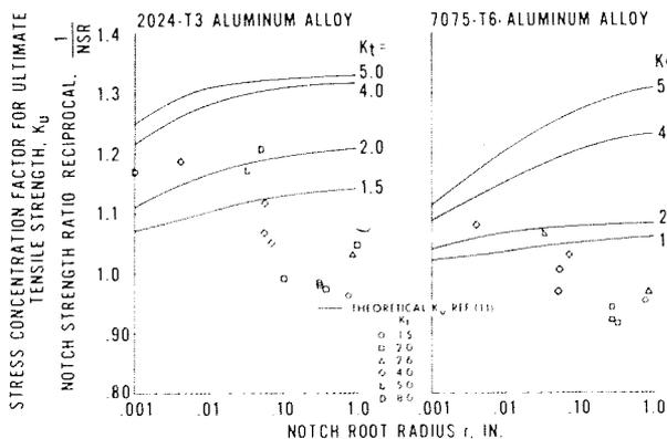
Fig. 10—Comparison of notch strength with theory based on cracked specimens
