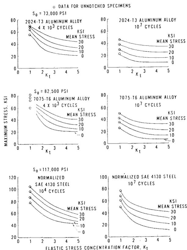
Fig. 3—Stress variation with stress-concentration factor for constant mean-stress curves
