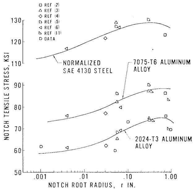
Fig. 8—Notch-tensile-strength vs. notch-root radius for all values of elastic stress-concentration factors
