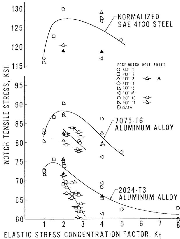
Fig. 6—Notch-tensile-strength variation with stress-concentration factors
