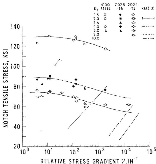
Fig. 9—Effect of relative stress gradient on the notch strength
