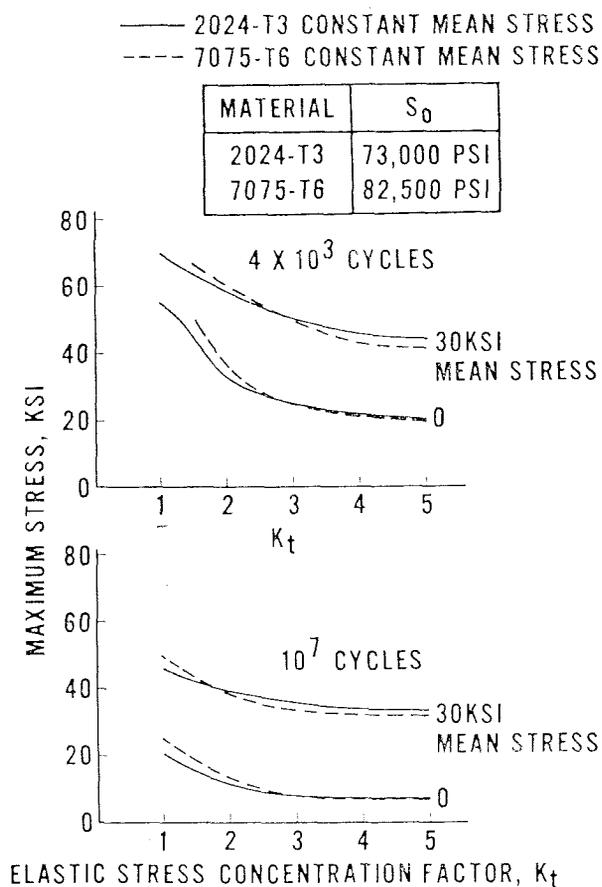
Fig. 4—Comparison of fatigue life of 2024-T3 and 7075-T6 aluminum alloys
