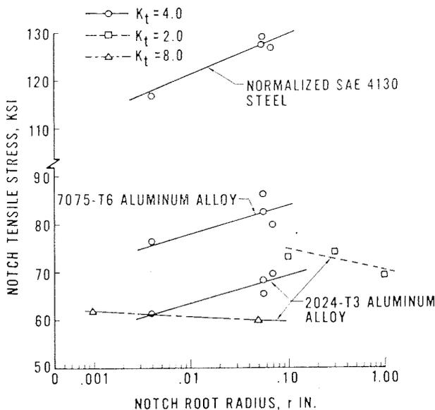
Fig. 7—Notch-tensile-strength variation with notch-root radius for constant elastic stress-concentration factor
