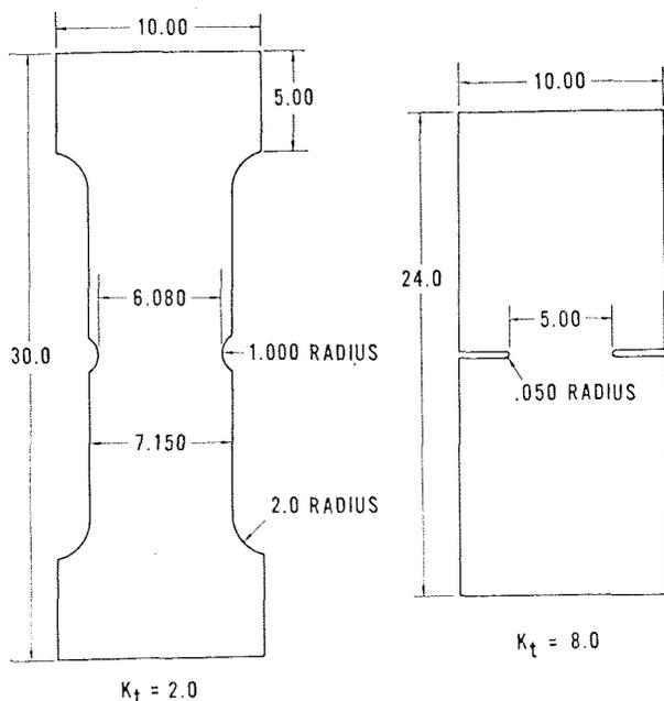
Fig. 2—Configuration of sheet specimens
