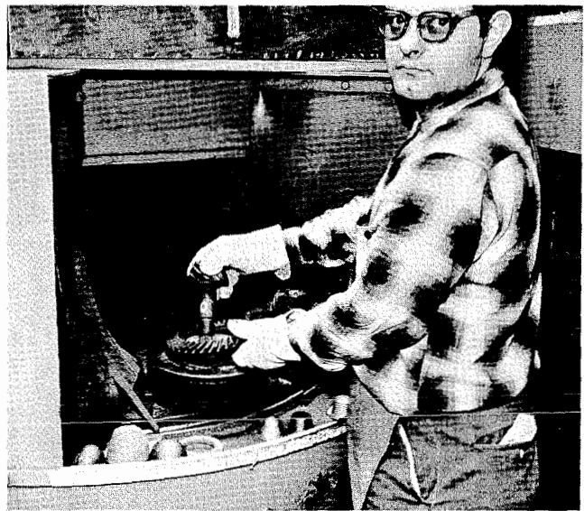
Figure 9 — Loading matched set of Bevel Gears on Multi-Table Machine.
