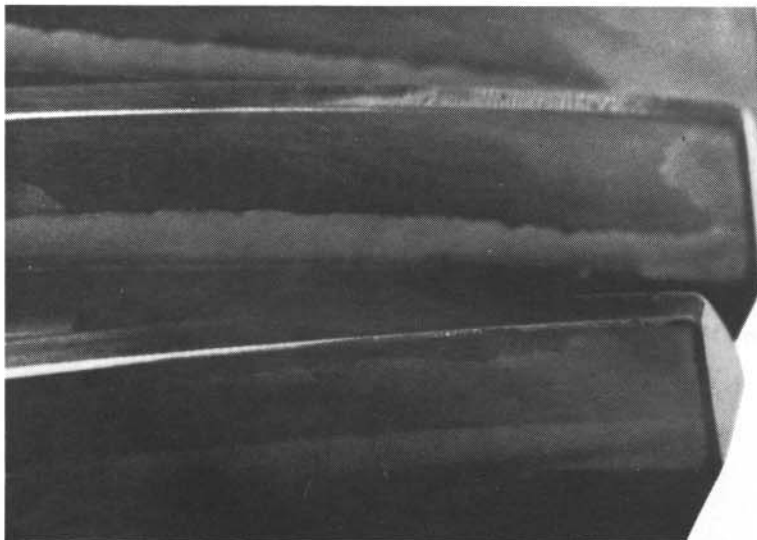
Frosting: This hardened helical gear shows a typical frosting pattern. Note that frosting is predominantly in the dedendum section, although patches do appear in the addendum section. This frosting pattern shows no radial welding and tear marks.
