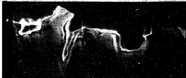
Fig.6: Shot peening of Aluminium precoated with PE coat.
