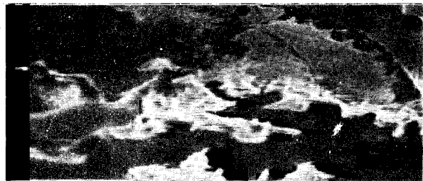
Fig.7 Shot Peening of Aluminium precoated with PE: No cracks.
