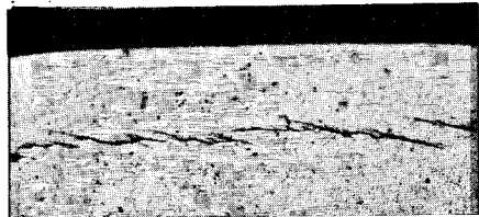
Fig.5. Crack nucleating in subsurface after shot-peening.
