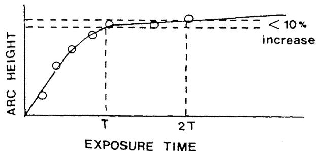
Figure 1. Determination of Almen saturation
