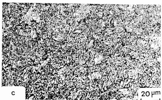
Figure 2. Microstructure of (a) test gear tooth (b) tooth case (c) tooth core
