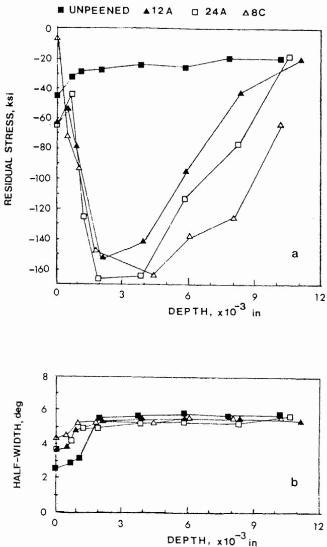
Figure 6. (a) Residual stress and (b) (211) peak width distributions of unpeened and peened gears
