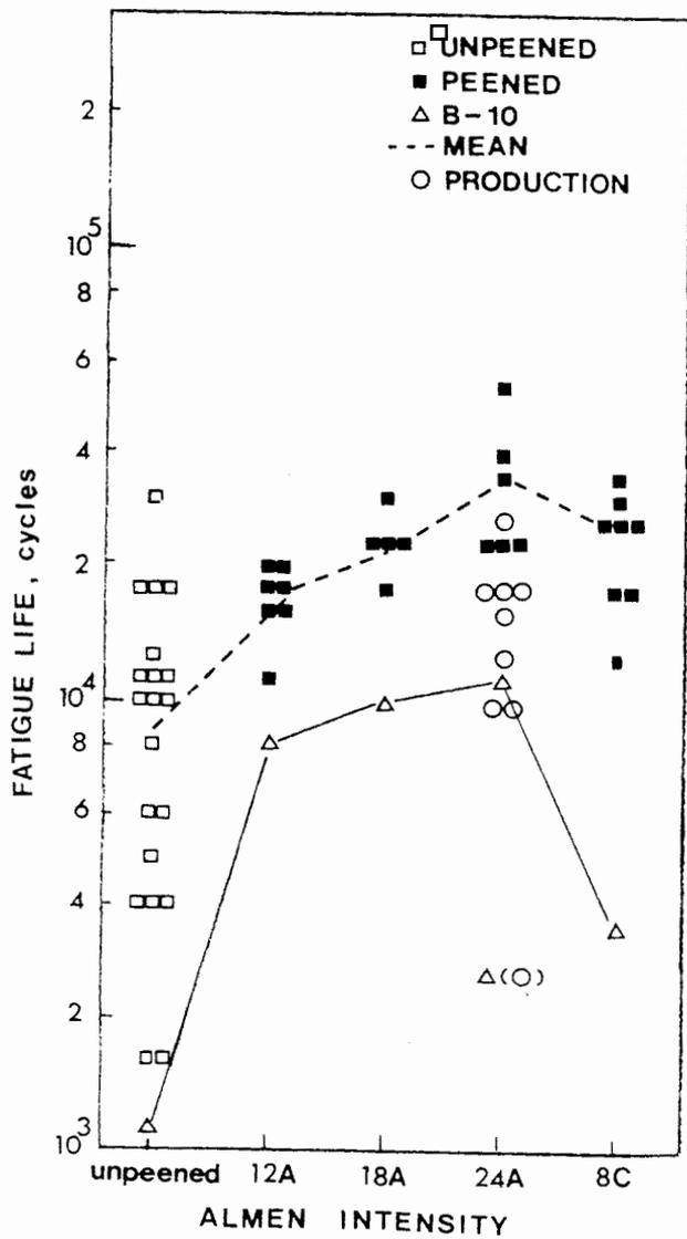
Figure 5. Effect of Almen intensity on fatigue life
