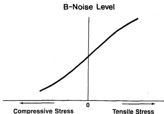
FIGURE 1 Barkhausen noise level as a function of stress in the elastic region.
