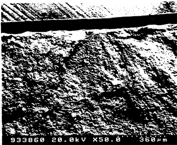
Fig. 11: Crack growth from the surface (Condition 'CP')
