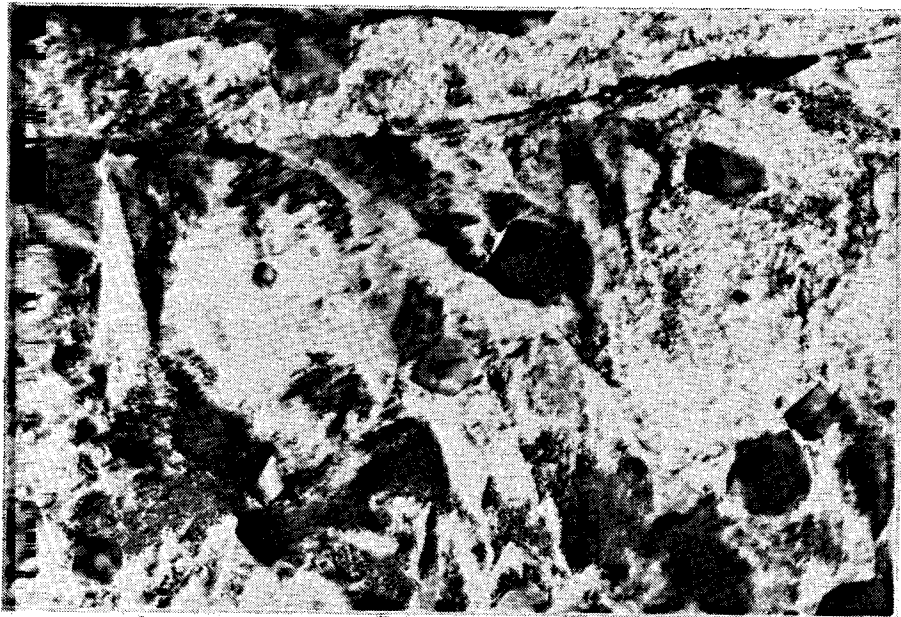
Fig.4 Structure of steel before plastic strain - austenite areas well seen multiplied x 42 000.
