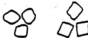
2. Unacceptable Shapes; Partially and Unconditioned Cut Wire Shot
