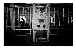
patterns on Glass sheets by blast-etching. The machine is simple to operate with minimum maintenance. One operator has to simply load and push the Glass sheets on idler rollers (inclined at a certain angle to vertical) into the cabinet. Another operator manually uses the blasting gun to etch the glass sheet as per the stencil (Stencil is in buyer's scope).
