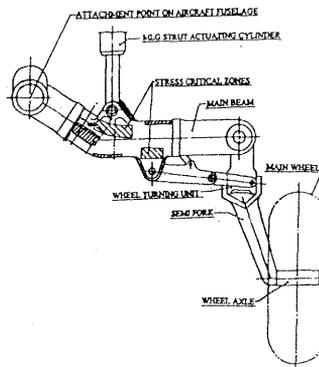
Fig. 1 MAIN LANDING GEAR STRUT
