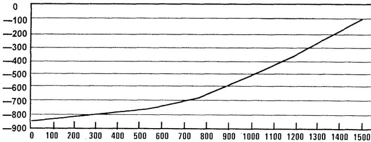
Fig. 5 Residual stress Vs No. of Landings
