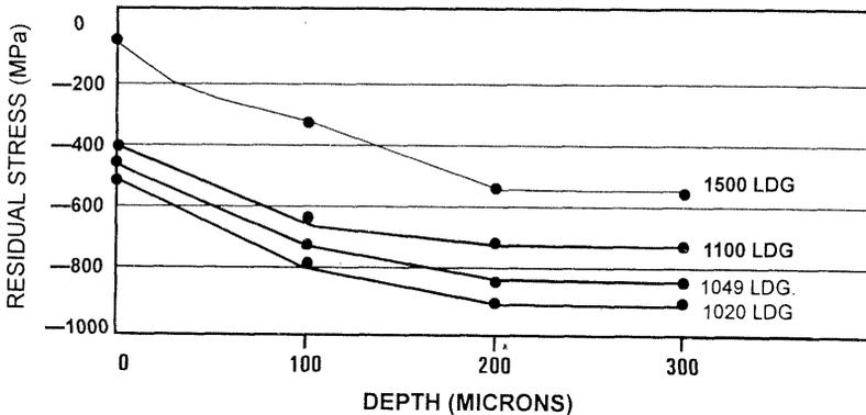
Fig. 6 Residual stress Vs Depth
