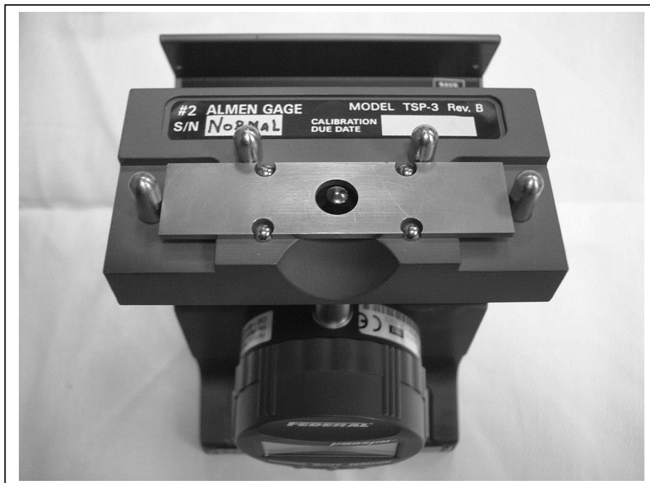
Figure 3. Special template to verify position of 4-balls
