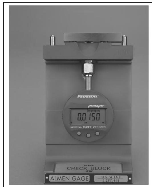
Figure 2c. Step block to right for calibration (inch mode)
