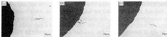
Figure 3. HIC initiation sites at: (a) mode I notch tip; (b) combined I/II mode ( K_{II}/K_I = 3.1 ) slit tip (in SSRT tests); (c) combined I/II mode ( K_{II}/K_I = 3.1 ) slit tip (in CLT tests).
