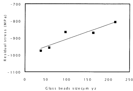
Figure 6: Relationship between residual stress and glass beads size, pressure 0.7\ \text{MPa}
