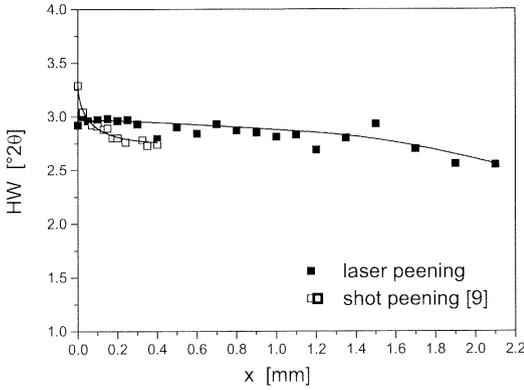
**Figure 4:** Half width depth distribution of laser peened and shot peened samples of AISI 4140
