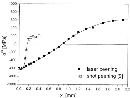
**Figure 3:** Residual stress depth distribution of laser peened and shot peened samples of AISI 4140
