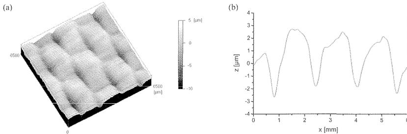
**Figure 1:** Surface structure (a) and profile line (b) of AISI 4140 after laser peening with two overlapping (50 %) layers
