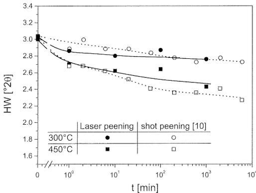
**Figure 6:** Measured thermal half width relaxation at the surface of laser peened and shot peened samples
