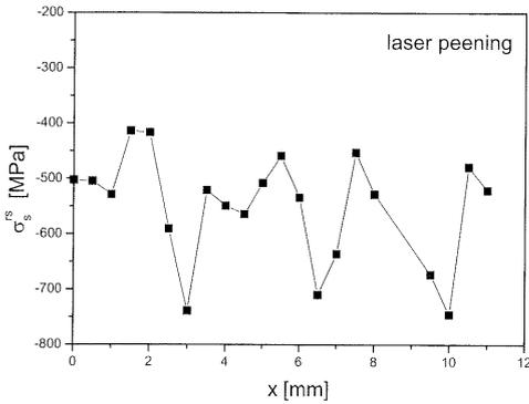
**Figure 2:** Surface residual stresses after laser peening with two overlapping (50 %) layers
