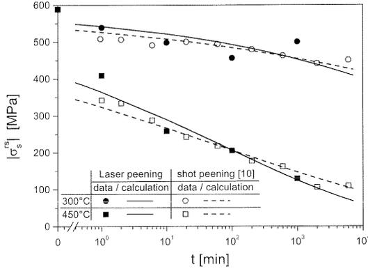
**Figure 5:** Measured and calculated thermal residual stress relaxation at the surface of laser peened and shot peened samples
