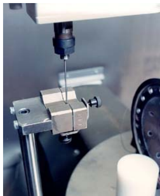
Figure 30 – PROGRESSIVE's small hole Almen tooling. A range of hole sizes are available.
