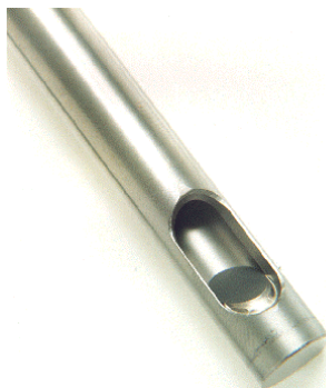
Figure 21 – Closeup of deflector and exit geometry
