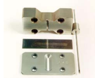
Figure 31 – Mask plate for 0.14" hole, simulated hole fixture, peened strip and small rotary lance.
