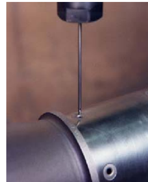
Figure 22 – Peening a turbine shaft oil hole (0.140" diameter)
