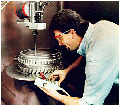
Figure 15 – PROGRESSIVE Rotary Lance Drive mounted on a PROGRESSIVE robot
