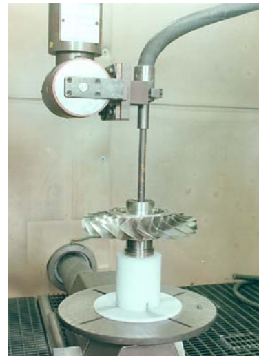
Figure 14 – A deflector used for peening a blisk bore.
