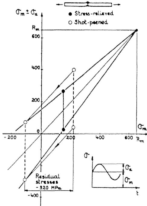
Figure 12 – Influence of a static stress on the fatigue limit of butt welds E 490 steel (MAG welding process) [ 15] .
