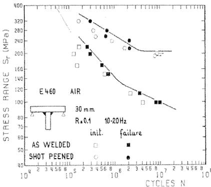
**Figure 3 – Fatigue strength of weld joints in steel E460 in as welded ar the shot peened conditions**
