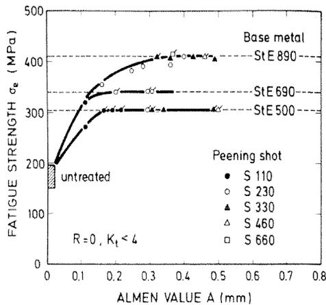
Figure 7 –Almen value vs. fatigue strength of butt weld [ 13]
