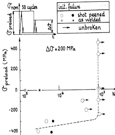
**Figure 8 – Influence of high stress peaks (tensile or compressive preloading) on the fatigue life of a welded shot peened joint in E460.**
