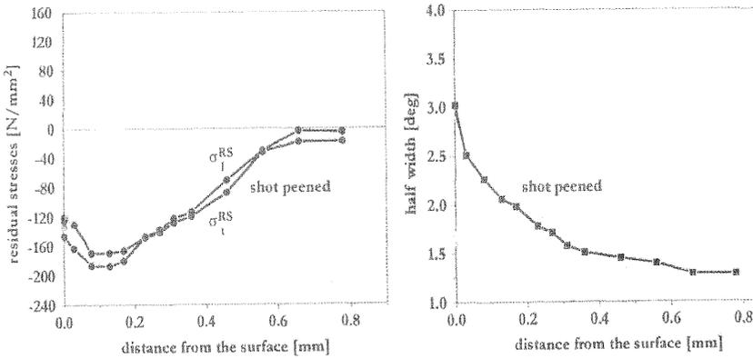
**Figure 1 – In depth characteristics induced by shot peening in a aluminium alloy butt welded joint [ 2 ]**
