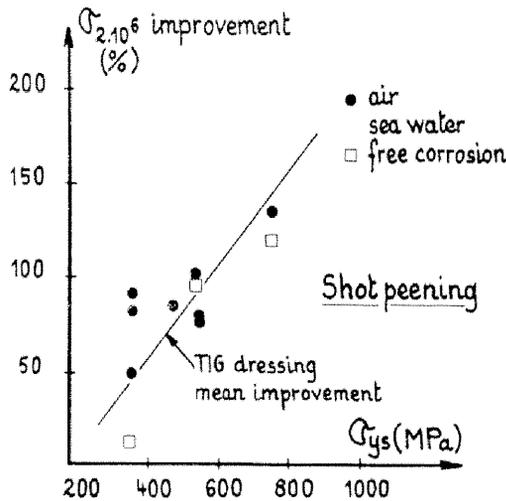
Figure 4 – Influence of base metal yield strength on the fatigue strength improvement by shot peening [ 10 ]
