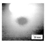
Figure 5: Roughened aluminum surface
