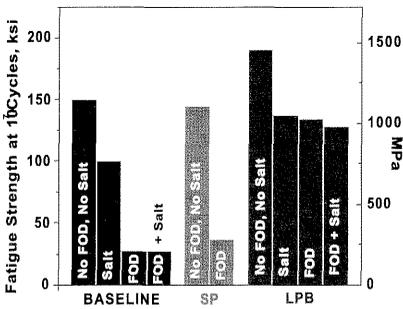
**Figure 7** HCF and corrosion fatigue of 17-4 PH stainless steel.
