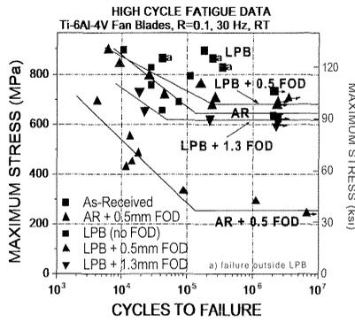
**Figure 6** - Effect of LPB in mitigating HCF and FOD damage in Ti-6-4 fan blades.
