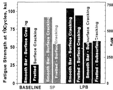
**Figure 8** - Ti-6Al-4V fretting fatigue data for shot peened and LPB surface treatments.
