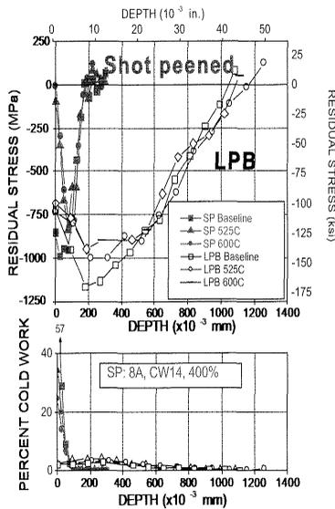
**Figure 4** – Thermal relaxation of surface treated IN718 showing relaxation in highly cold worked layers.
