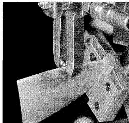
**Figure 2** LPB treatment of LE of 17-4PH compressor blade with caliper tool.
