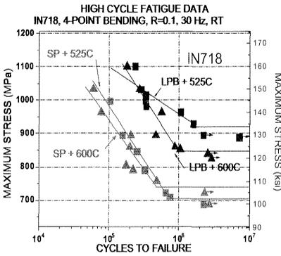
**Figure 5** - High cycle fatigue performance of surface treated IN718.
