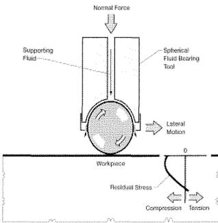
**Figure 1** LPB Schematic showing constant volume ball support and separately controlled normal force.
