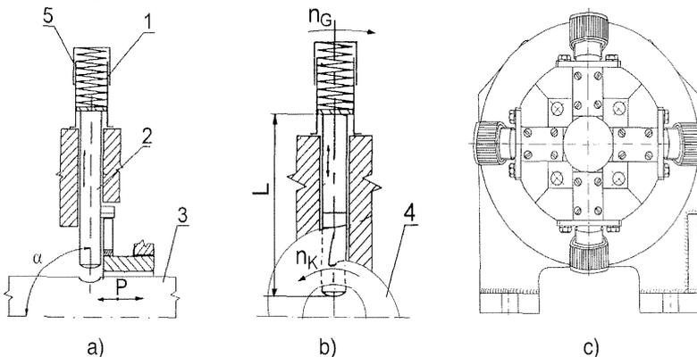
Fig. 2. Scheme of the percussive device for percussive burnishing process: a) mechanism elements and processed shaft, b) mechanism with the cam, c) percussive burnishing head; 1 - spring, 2 – percussive element, 3 – processed shaft, 4 – cam, 5 - adjusting nut,  $n_K$  – cam rotation speed,  $n_G$  – head rotation speed, L – length of percussive element,  $\alpha$  - striking angle
