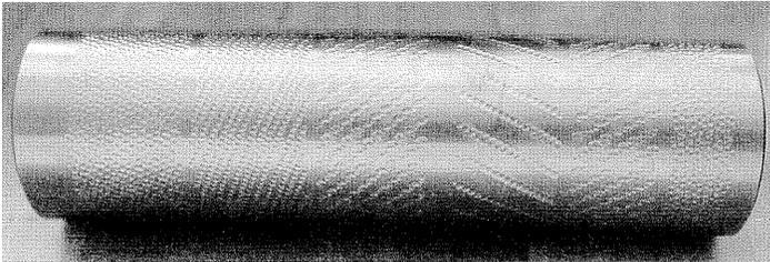
Fig 3. Photo of the surface after the percussive burnishing process
