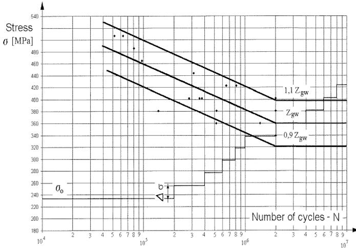
Fig. 5. Wöhler curve;  $\sigma_0 = 234$  MPa,  $\Delta\sigma = 21$  MPa,  $n_i = 2 \cdot 10^5$  cycles
