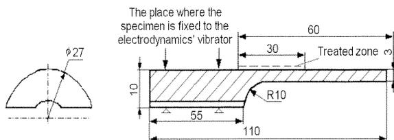
Fig 4. Shape and dimensions of the samples for fatigue strength researches
