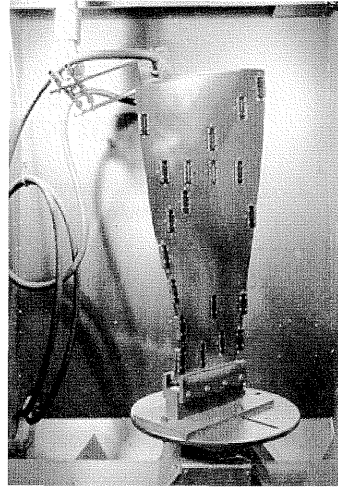
Figure 1 - This turbine engine fan blade has 40 Almen strip locations.
