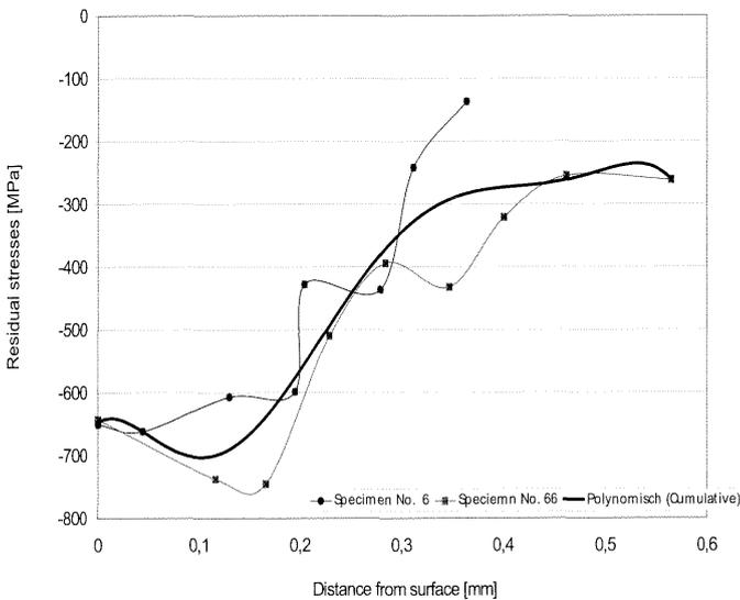
Fig. 2: Residual stress distribution after shot peening
