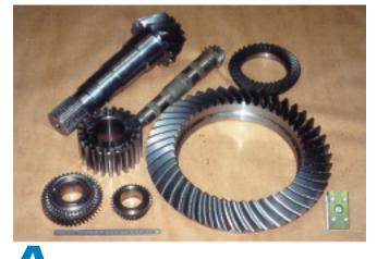
utomotive designers have traditionally relied on the advantages of shot peening of transmission parts to enhance their useful life. Commonly, shot peening machines are found post-heat treat and at the end of a production process for critical parts such as ring and pinion gear sets.
