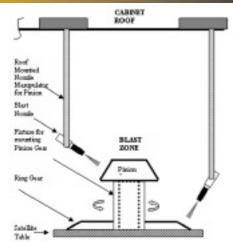
nozzle settings in order to achieve desired results on the pinion and ring gears.
