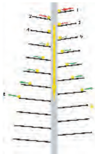
Fig.10 Schematic ‘tree’ of helix sections showing outward movement of a descending spherical shot particle.
