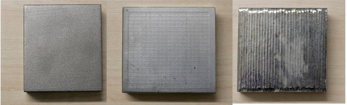
Shot Peened (SP)                      Laser Peened (LSP)                      Ultrasonic impact Peened (UIT)
