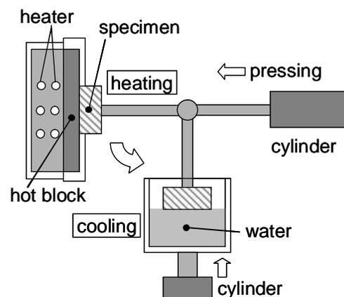
Fig.2 Schematic illustration of thermal fatigue test apparatus.
