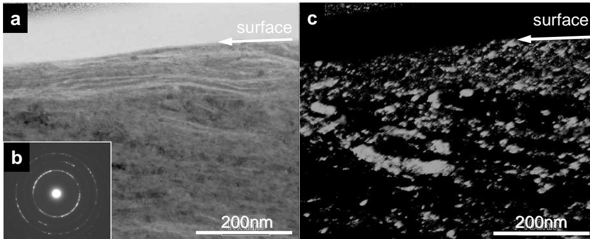
Fig.6 TEM micrographs of FPB'ed specimen. a), b) and c) are Bright field image, dark field image and selected area diffraction pattern, respectively.
