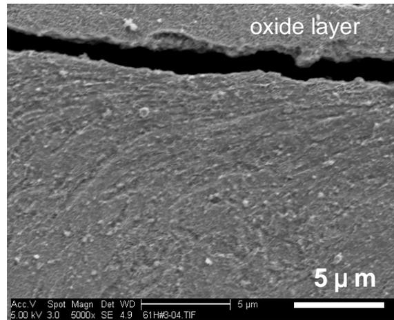
Fig.5 Cross sectional SEM micrograph of FPB'ed specimen after thermal fatigue test.
