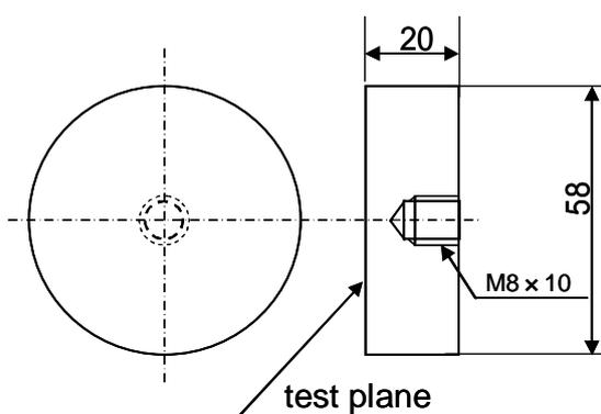
Fig.1 Size of specimen for thermal fatigue test.
