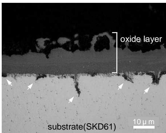
Fig.3 Typical heat cracks developed in as received specimen. The cracks are indicated by small arrows.
