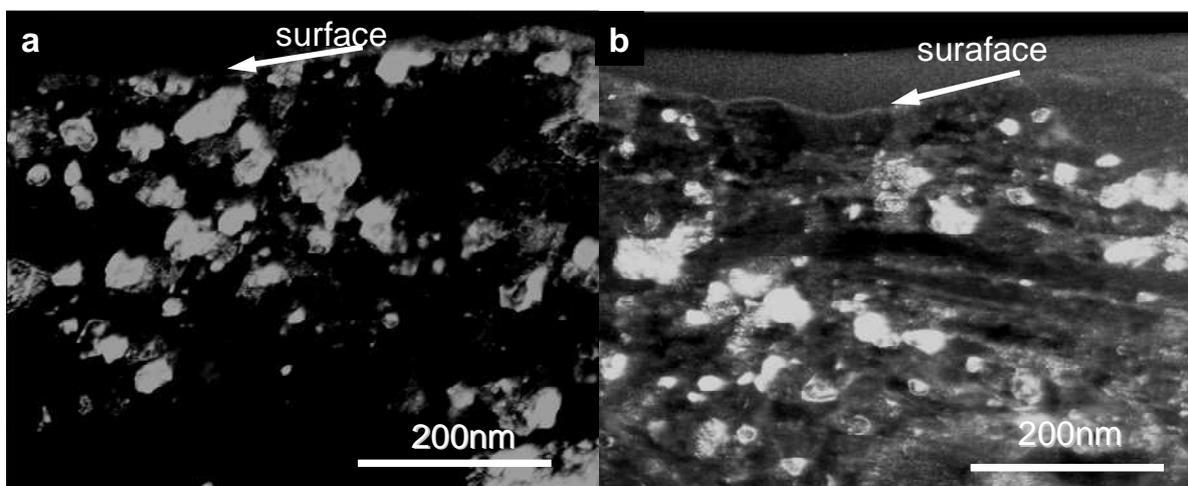
Fig.7 Dark field images by TEM. a) and b) are heat treated at  $843\text{K}$  and radical nitrated specimen, respectively.
