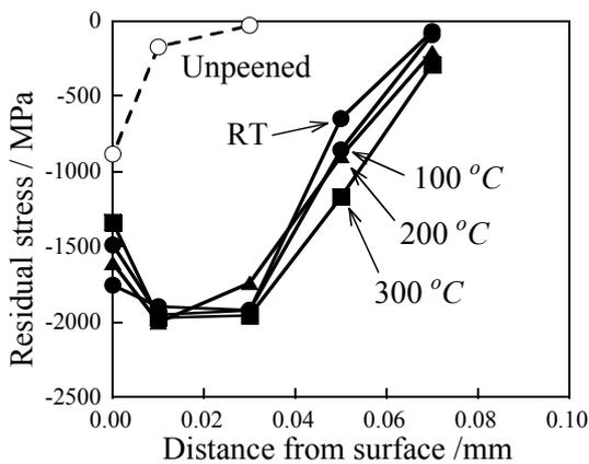
Figure 5 Distribution of residual stress in thickness direction in warm peening
