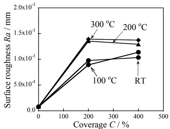
Figure 6 Variation of surface roughness with coverage in warm peening
