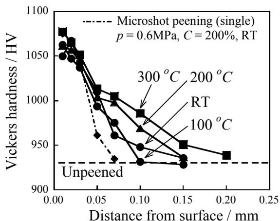
Figure 7 Distribution of Vickers hardness in thickness direction in warm double peening
