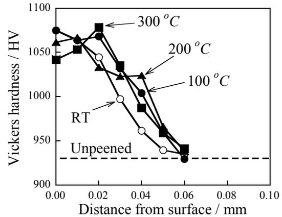
Figure 4 Distribution of Vickers hardness in thickness direction in warm peening
