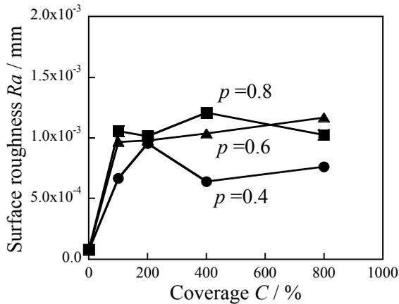
Figure 3 Variation of surface roughness with coverage in microshot peening
