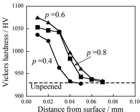
Figure 1 Distribution of Vickers hardness in thickness direction in microshot peening
