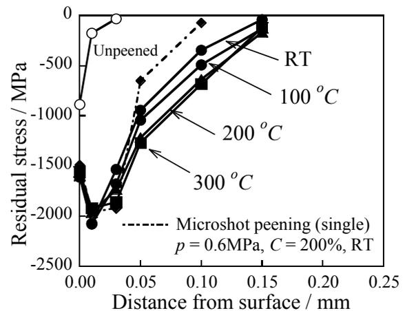
Figure 8 Distribution of residual stress in thickness direction in warm double peening
