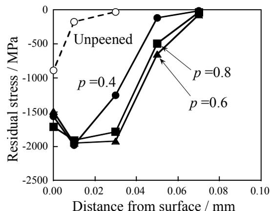
Figure 2 Distribution of residual stress in thickness direction in microshot peening
