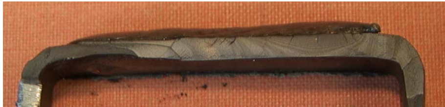
Figure 7 Typical variable amplitude fatigue fracture surface, VA3 spectrum laser peened
