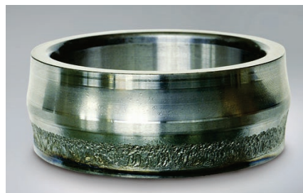
Figure 1. Flaking on the Bearing Raceway Surface
