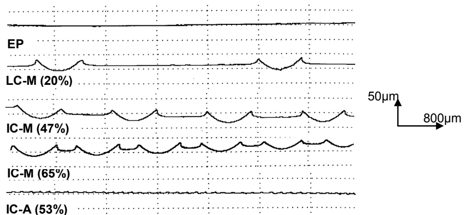
Figure 4: Surface roughness profiles of the various conditions (225bar BB-pressure)
