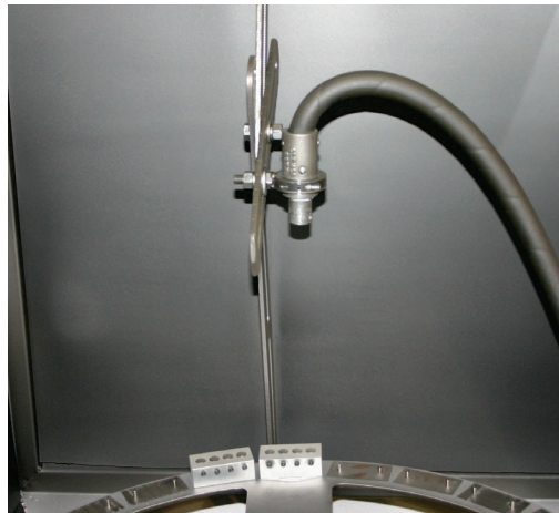
Figure 3. Machine set-up showing nozzle standoff distance
