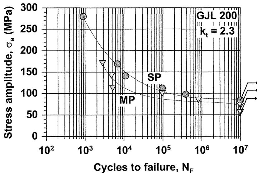
Figure 6 Influence of shot peening on the notched fatigue performance of GJL 200
