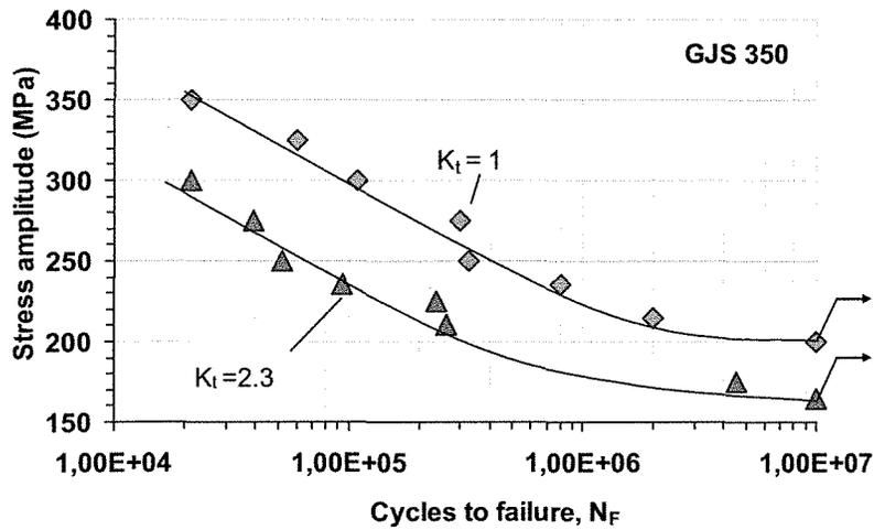
**Figure 9** Influence of notches on the fatigue performance of GJS 350
