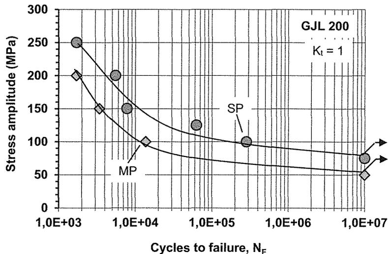
**Figure 4** Influence of shot peening on the smooth fatigue performance of GJL 200
