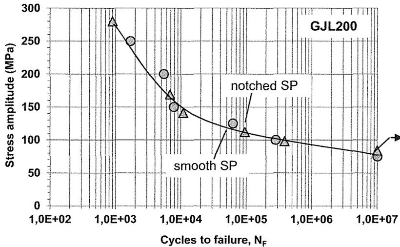
Figure 7 Comparison of shot peened smooth and notched specimens of GJL 200
