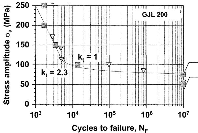
Figure 5 Influence of notches on the fatigue performance of GJL 200
