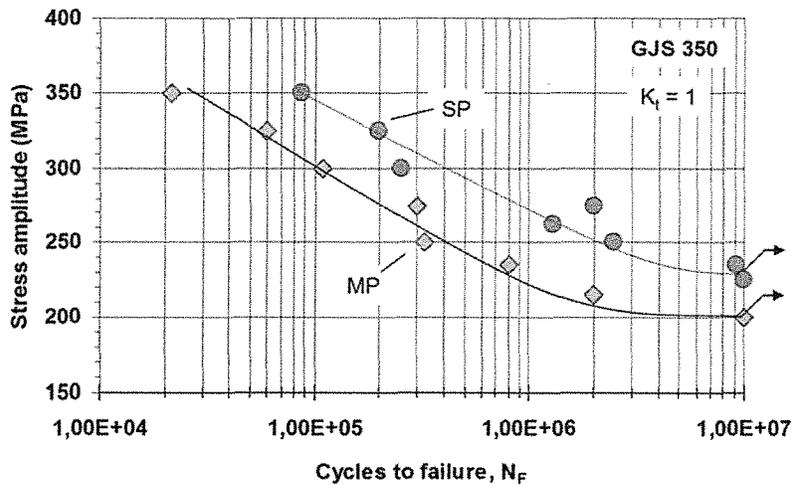
Figure 8: Influence of shot peening on the smooth fatigue performance of GJS 350
