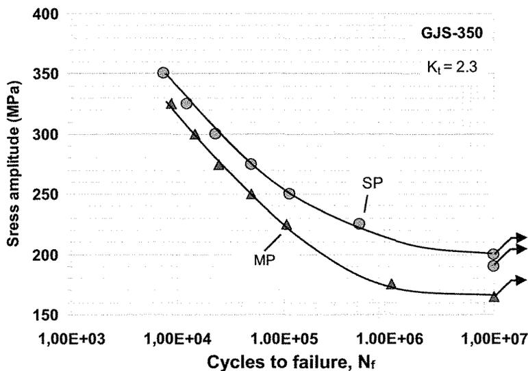
**Figure 10** Influence of shot peening on the notched fatigue performance of GJS 350
