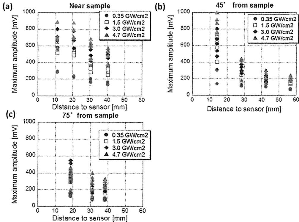
Fig. 3 Maximum amplitudes of detected AE events by laser ablation each sensor, (a) near the sample, (b) 45° from sample, (c) 75° from sample
