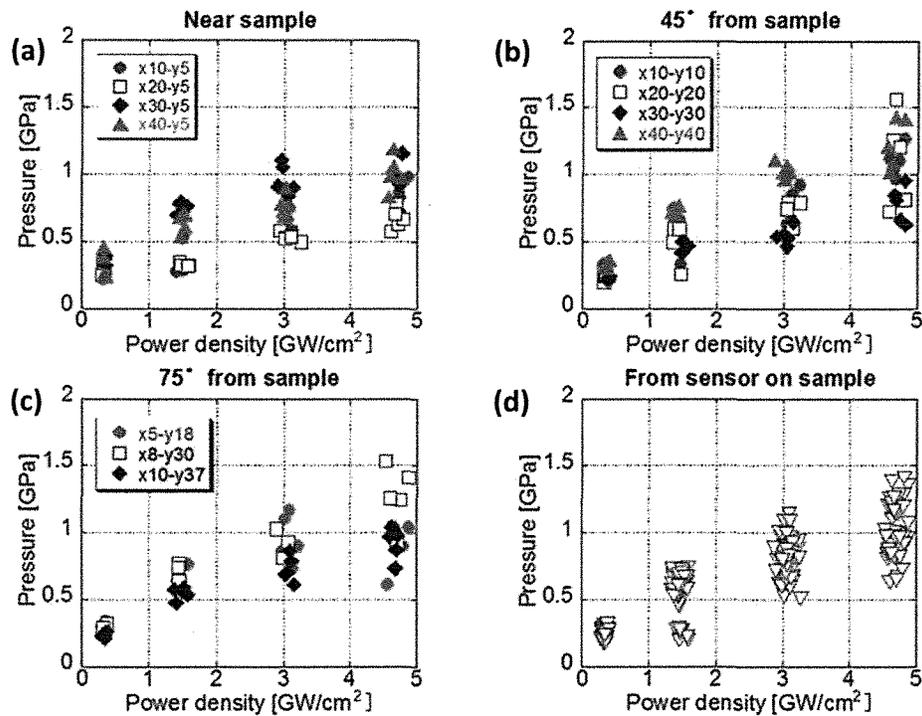
Fig. 4 Pressure by laser ablation each sensor, (a) near the sample, (b) 45° from sample, (c) 75° from sample, (d) on sample
