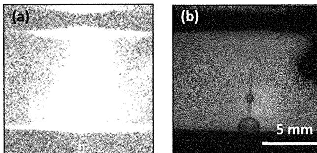
Fig. 5 High speed camera observation showing (a) laser-induced breakdown and (b) bubble formation after 26  $\mu$ s from laser irradiation
