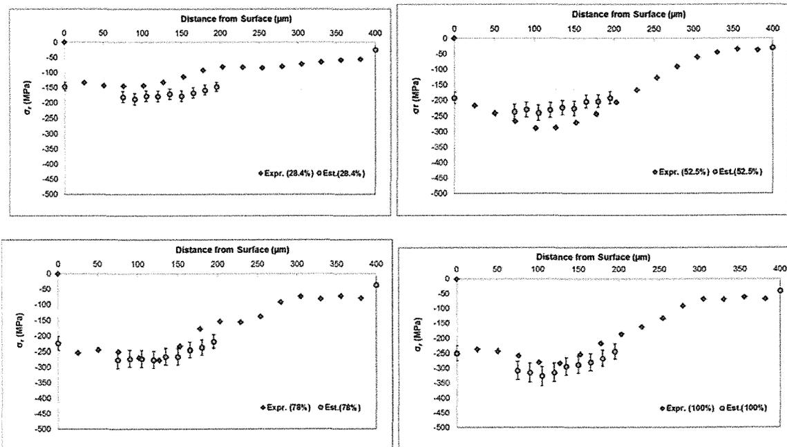
Figure 5 Estimation of the compressive residual stress from micro-hardness.
