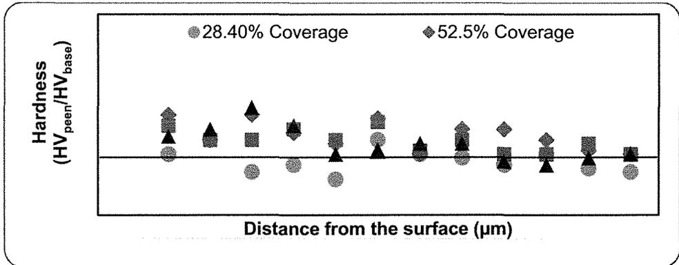
Figure 3 Normalized Hardness vs. distance from the edge surface ( $\text{HV}_{\text{base}} 100 \text{ g} = 160$ ).
