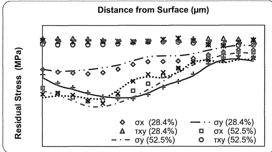
Figure 4 Stresses measured from Hole drilling method.
