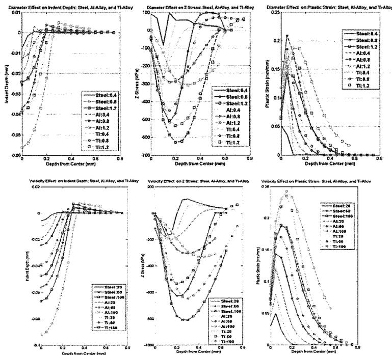
Figure 4: Effect of Shot Diameter and Velocity on Shot Peening (Steel/Al-7075/Ti-6Al-4V)
