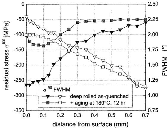
Fig.6: Residual stress and FWHM value depth profiles of differently treated materials states
