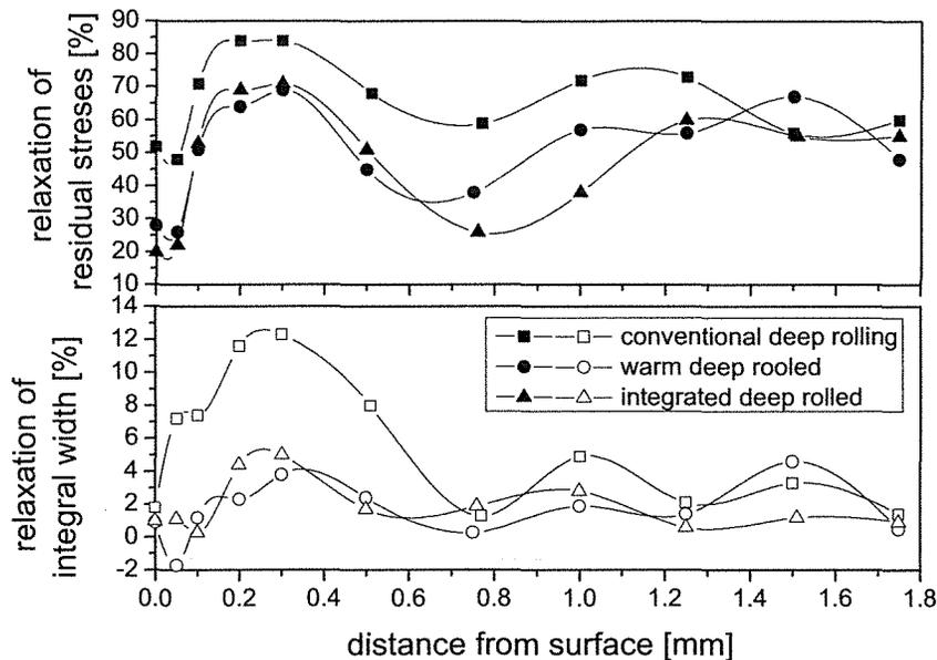
Fig. 3: Relative stability of residual stresses and integral width for different deep rolling procedures
