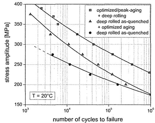
Fig. 7: S,N- curves of differently treated materials states
