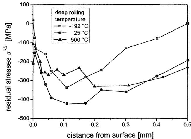
Fig. 10: Residual stress depth distributions (tangential direction) at different deep rolling temperatures
