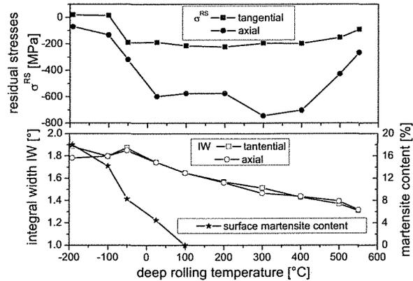
Fig. 9: Surface residual stresses (above) and integral width and martensite content (below) after deep rolling at different temperatures
