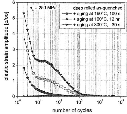
Fig. 5: Cyclic deformation curves of differently treated materials states
