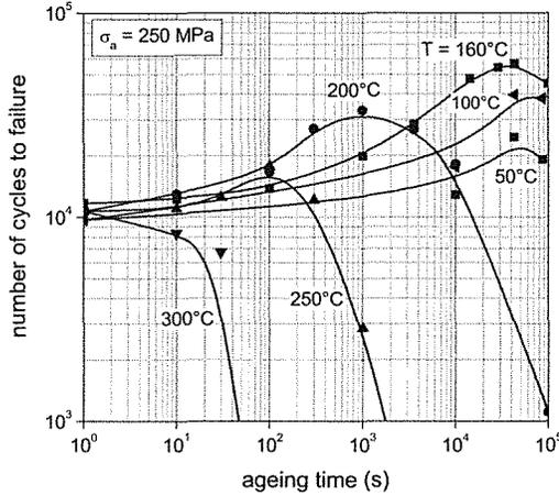
Fig. 4: Fatigue lifetime as a function of aging time and temperature [10]
