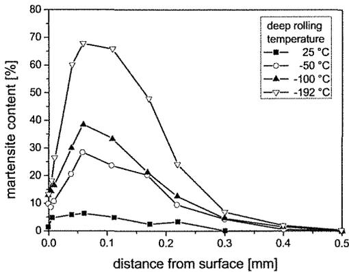
Fig. 8: Depth distribution of martensite content after different deep rolling treatments [11]
