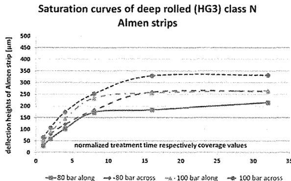
Fig. 6: Saturation curves of deep rolled (HG 3) class N Almen strips
