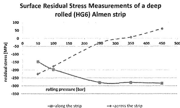
Fig. 10: Surface Residual Stress Measurements of a deep rolled (HG6) Almen strip
