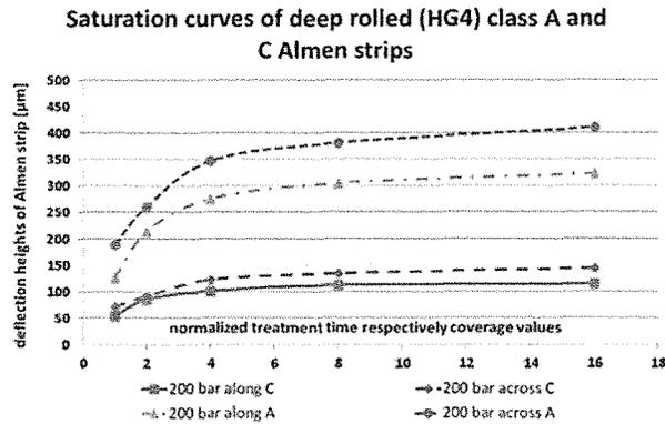
Fig. 9: Saturation curves of deep rolled (HG 4) class A and C Almen strips
