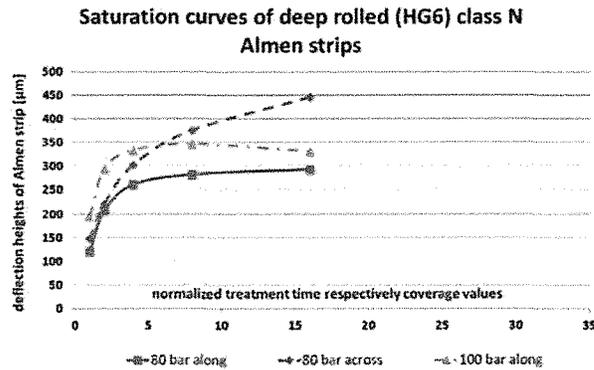
Fig. 7: Saturation curves of deep rolled (HG 6) class N Almen strips
