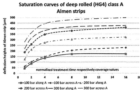
Fig. 8: Saturation curves of deep rolled (HG 4) class A Almen strips
