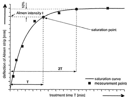
Fig. 2: Deflection of an Almen strip in dependence of the treatment time (FE12: 33)
