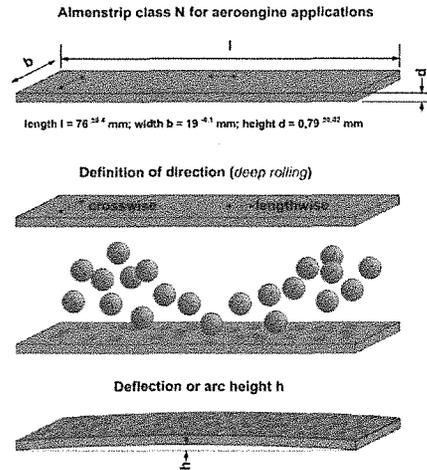
Fig. 1: Schematic view and definitions of Almen strips and their parameters (FE 12: 32)
