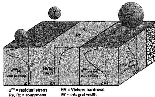
Fig. 4: The characteristic parameters concerning shot peening and rolling. (FE 12: 34)
