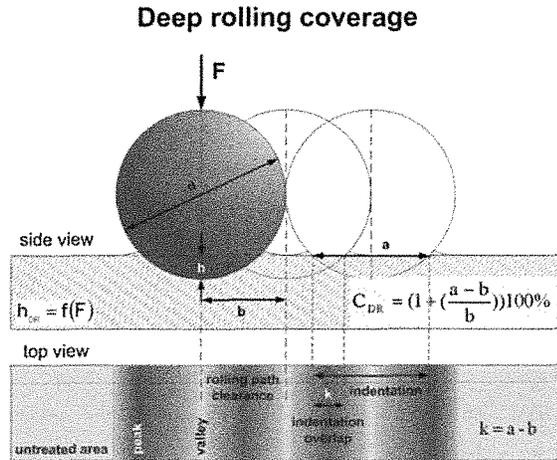
Fig. 5: Additional factors which characterise the deep rolling process (FE 12: 40)
