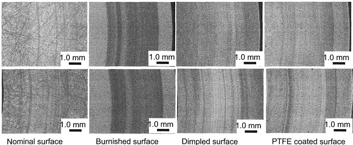
Fig. 8 Optical image of raceway of bearing ring (upper) and washer (bottom)
