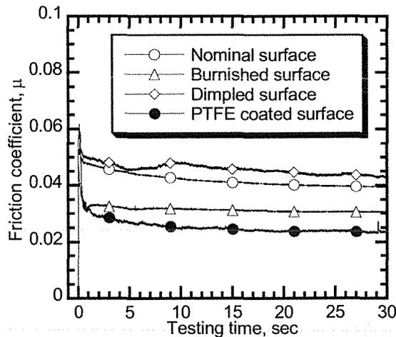
Fig. 9 Friction coefficient vs. testing time
