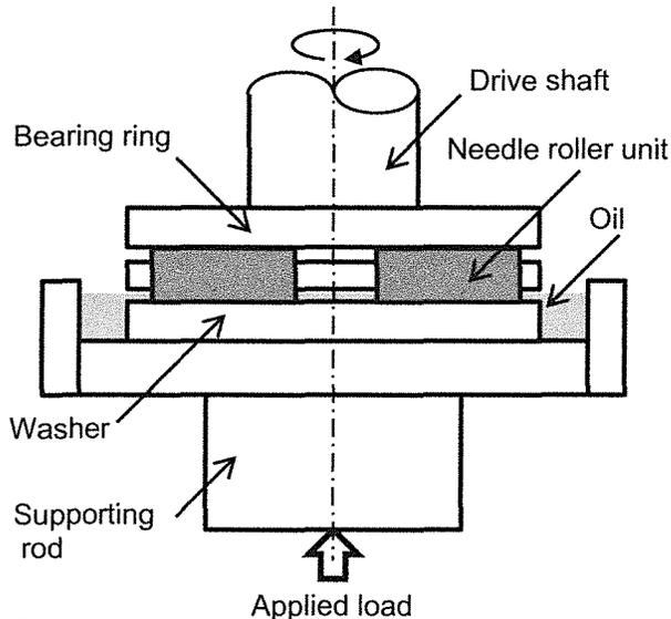
Fig. 6 Schematic of Rolling sliding apparatus
