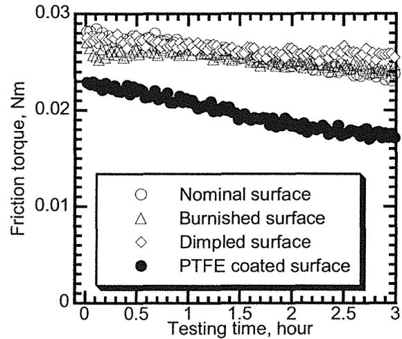
Fig. 7 Friction torque vs. testing time
