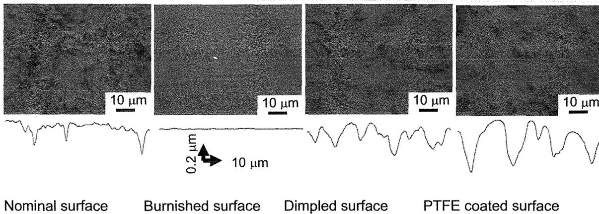
Fig. 5 Optical micro image and surface profile of bearing ring and washer surface
