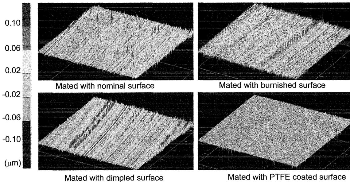
Fig. 11 3-D Surface profile of ring surface mated with dimpled and PTFE coated surface
