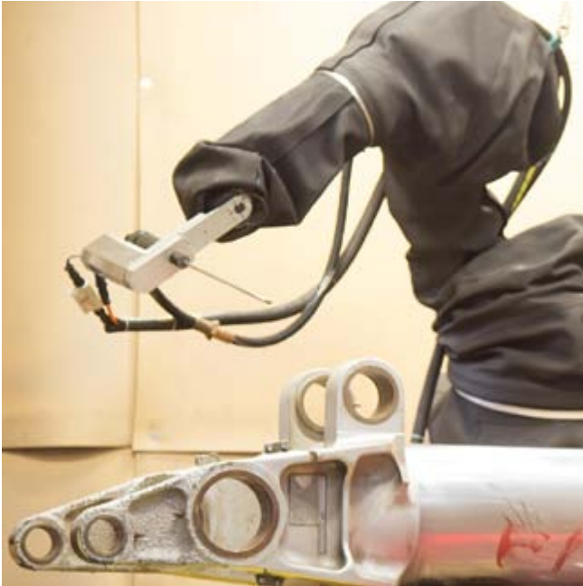
Robotic manipulator featuring the rotary nozzle system
