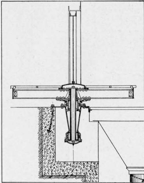
Section of Blast Room Showing Standard Pedestal Type of Rotary Table.
