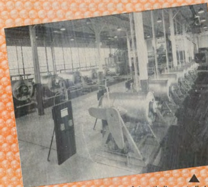
▲ Automatically controlled heat-treating equipment assures a non-varying metallurgical structure of tempered martensite for long life and economical cleaning.
