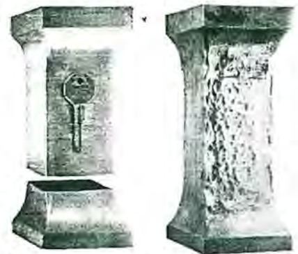
Fig. 15—Non-peened and hammer peened reverse bending fatigue specimens made of SAE 1030 annealed steel that were used in a study of forge hammer base failures.
