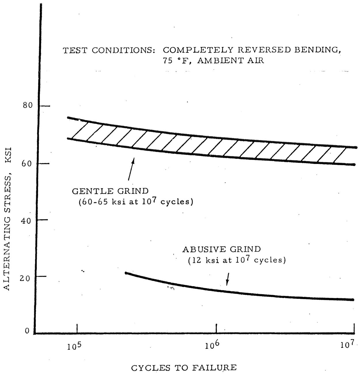
Figure 1 - FATIGUE CHARACTERISTICS OF ANNEALED
